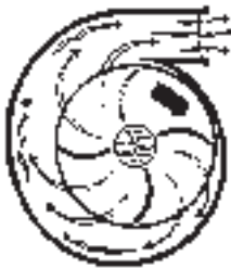
Centrifugal Pump — Variable Torque Load
