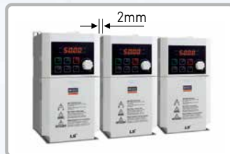
Side-by-side Installation (2mm between drives)
